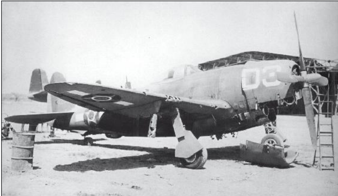
Damage caused to Perdigão's plane during his attack on 24 April when he passed through the ball of fire from the explosion of his target. (Author's collection)
