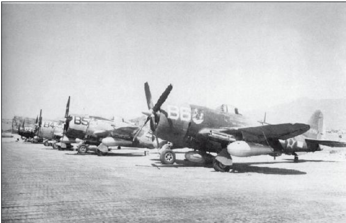
yellow escadrille line up with rocket launchers and incendiary bombs built using 75-gallon fuel tanks. (Author's collection)
