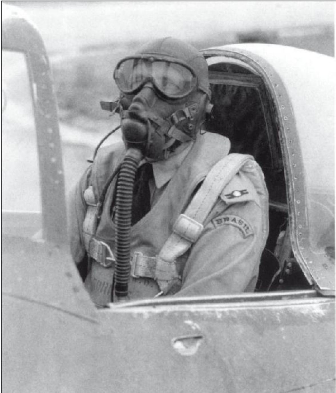
The oxygen mask was widely used because of the high cruise altitudes en route to the targets and the risk of contamination from carbon monoxide. (Author's collection)
