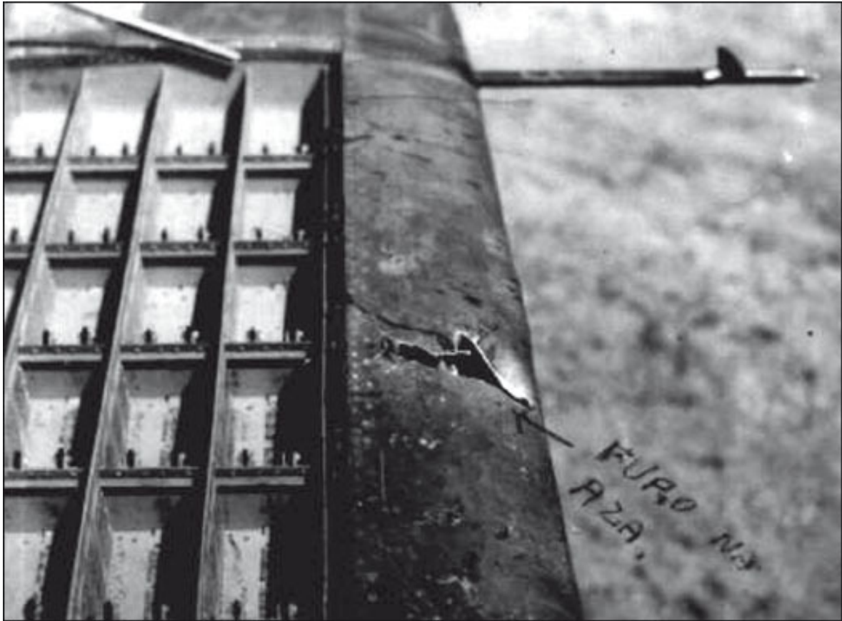
Damage to Perdigão's plane from his attack on 24 April when he passed through the ball of fire from his exploding target. (Author's collection)
